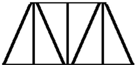
A bridge consists of trusses on the sides, as well as a deck on the bottom. To avoid a collapse at the top, you should include bracing at the top, again consisting of triangles like the first figure. You should line up vertical joints exactly with horizontal joints to avoid "punch through". There should also be **lateral bracing** at the top, to avoid shear in the transverse structure.
