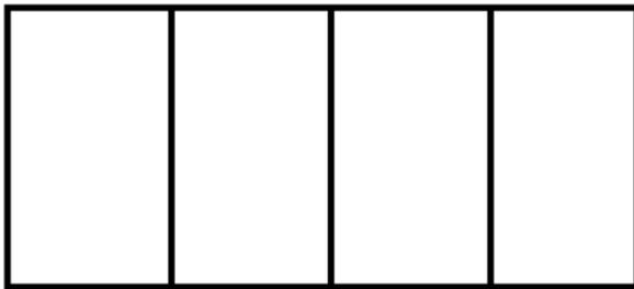
This bridge will resist bending, but will be very vulnerable to shear. We use trusses [diagonals] to handle shear forces efficiently.
