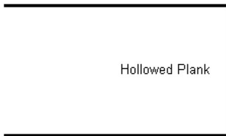
However, in such a case, the **top** part of the beam would carry **all the load**, and the **bottom** part would support **nothing**. Therefore, we insert vertical supports to transfer the load from the top to the bottom:
