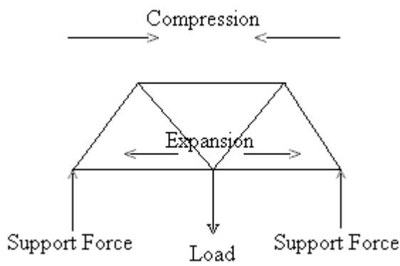
The effect of the load, and the balance of "bending moments" [what Civil Engineers call "torques"] results in compression on the top members, and forces of expansion at the bottom.
