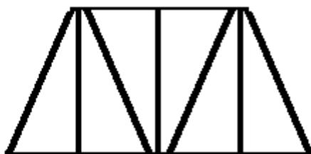
The two good things about trusses are (1) that they can handle shear forces efficiently, and (2) that truss bridges --- assuming ideal "pin connections" --- are completely solvable, as well as generally strong structures. Note that the "triangulation" provides strength by preventing "buckling" of the bridge. [Since the ends of the bridge are supported by the abutment and do not experience a bending moment, a triangular portion at each end, being unnecessary, is removed.]
