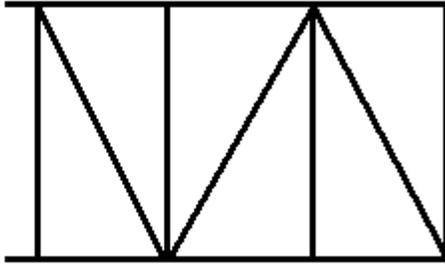
**Craftsmanship is important** in preparing these joints, in that it is important that the pieces fit together tightly, and that the joint members line up so that their centers meet at a point. The fundamental principle of Truss Design is to replace all **shear** and **bending** forces with **compression** and **extension** forces, and to reduce the structure to a **series of triangles**. There are several different types of basic bridge designs, such as these:
