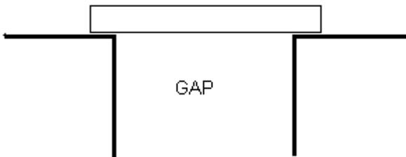
This is not a very good bridge design, as can be seen in the "worst case" scenario by putting a significant load at the middle of the bridge. The bridge will bow in the middle if the load is substantial enough, because of the **Shearing Force** and the **Bending Moment**.
