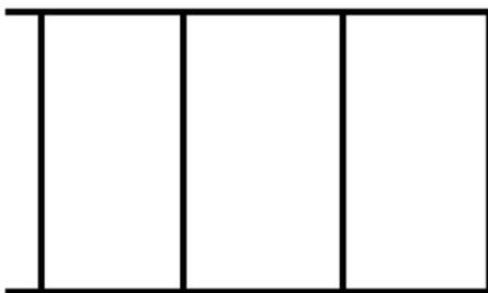
The **shear forces** would then cause a problem, and we must add diagonal members to transfer **both horizontal and vertical forces**. It is the **vertical components** that serve to reduce **shear forces**:
