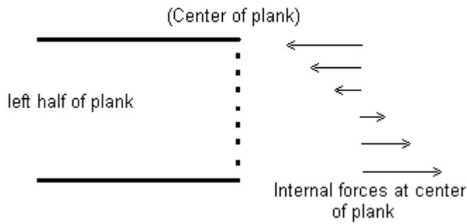
From an engineering viewpoint, the material along the edges of the plank is under the greatest distress [stress], so that it would constitute an improvement to "hollow out the beam":
